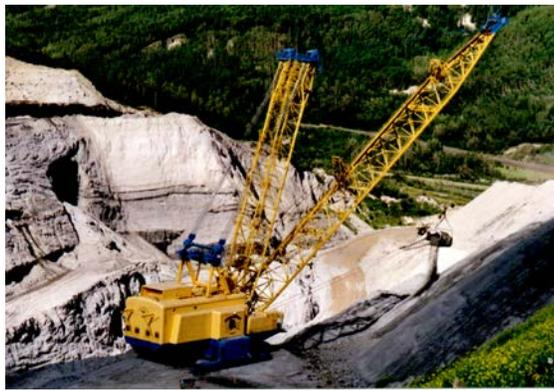
The dragline has a total weight of more than 2,200 tons. The dragline buckets move 33 to 37 cubic yards of material. The crew consists of two operators that rotate positions every hour. When they aren't at the controls, they do maintenance and repair. The dragline is electrically powered through a large cable connected to the utility power system.
